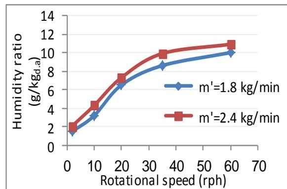
Fig.12. Effect of the rotational speed on the outlet humidity ratio of process air at different air flow rates during adsorption process at a regeneration temperature of 110o C
