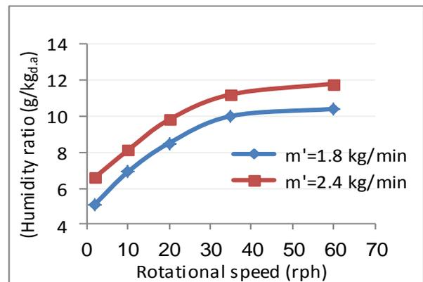
Fig.13 Effect of the rotational speed on the outlet humidity of process air at different at air flow rates during adsorption process at a regeneration temperature of 800 C
